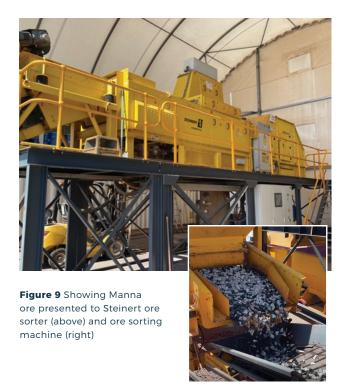
The ore sorter results show the trial successfully reduced the gabbro/basalt diluted component reducing the iron in the feed from  $6.3\%~Fe_2O_3$  to  $0.4\%~Fe_2O_3$ . Lithium chemical plants typically request a final spodumene concentrate iron specification <1% Fe<sub>2</sub>O<sub>3</sub>.
