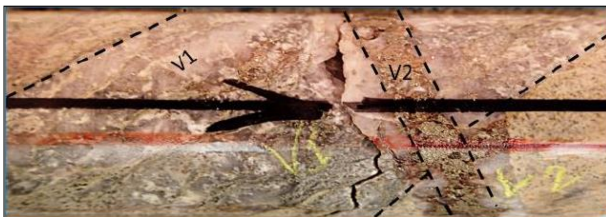
Figure 9: Thin pyrite-rich V2a vein crosscutting obliquely a quartz-carbonate-pyrite V1 vein, MSDD007, 260 m.
