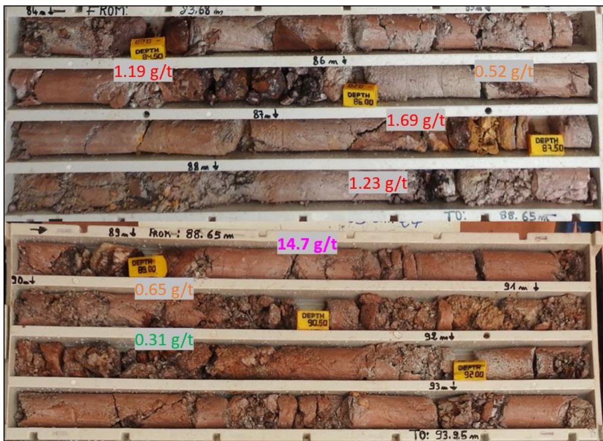
Figure 12: MSDD007 drill core with assays displayed, 7m @ 2.9 g/t gold
