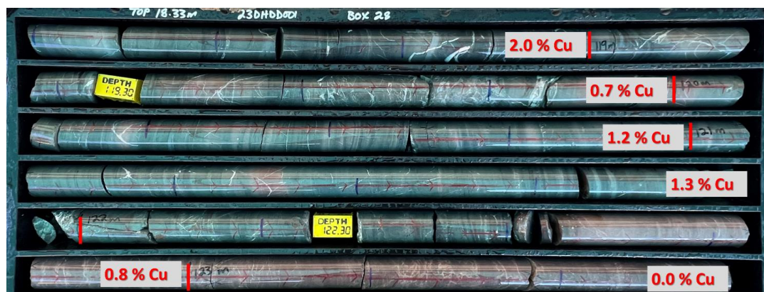
Figure 11: Drill core from 23DHDD001 showing bedded siltstone units with brittle fractures and Quartz-Carbonate veining with chalcopryrite and chalcocite mineralisation from 118-123m.
