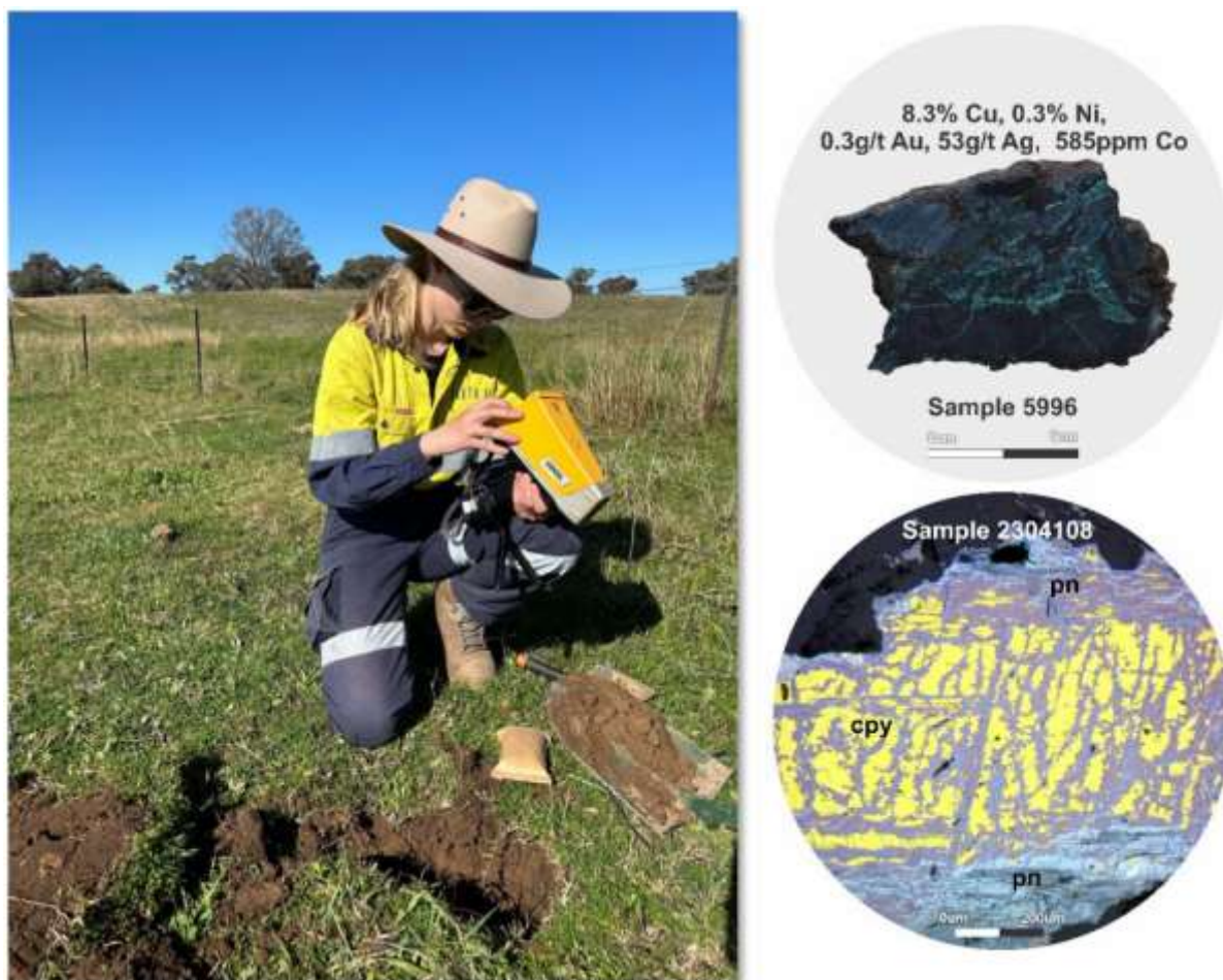
FIGURE 9: EARTH AI FIELD TEAM CONDUCTING SOIL SAMPLING AT FONTENOY (LEFT), AND ROCK SAMPLE 5996 (TOP RIGHT), AND NICKEL SULPHIDES (PN - PENTLANDITE), COPPER SULPHIDES (CPY - CHALCOPYRITE) CONFIRMED IN SERPENTINITE/GABBRO THROUGH SEM AND PETROGRAPHIC ANALYSIS (BOTTOM RIGHT).
