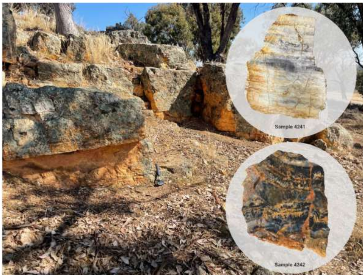
FIGURE 3: SINTER OUTCROP AT THE BRECCIA SINTER PROSPECT, AND INSERTS SHOWING SINTER RELATED LITHOLOGY SAMPLE 4241 OF THE BRECCIA SINTER PROSPECT AND SAMPLE 4242 FROM THE QUARRY PROSPECT. SAMPLES SHOW DOMINANT LIGHT AND DARK GREY CHALCIDONIC-QUARTZ BANDING WITH YELLOW TO LIGHT BROWN OXIDES AFTER POSSIBLE IRON-CARBONATE.
