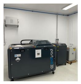
Singular 3DP invested in a vapor-fusing machine which is a critical postprocessing step for the preparation of patient-specific orthotics to create a smooth molded-plastic-like surface finish safe for the skin. With one of only two such machines in Australia, this also provides Singular 3DP with a sought-after supplementary service.
