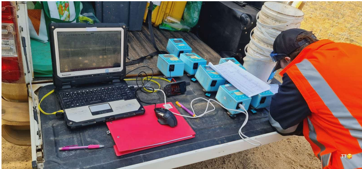
EMU's geologists working with Passive Seismic Survey recording equipment, Condingup WA
