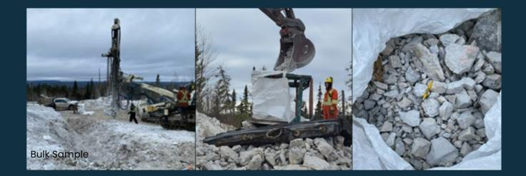
GTI has conducted diverse drilling campaigns, crucial for providing valuable information for the ongoing Preliminary Economic Assessment ('PEA'). These campaigns have primarily focused on gathering geotechnical data, utilising exploration diamond rigs onsite. The scope of these campaigns included condemnation (sterilisation) diamond drilling and bedrock mapping, covering all areas where major infrastructure is proposed to be situated.
