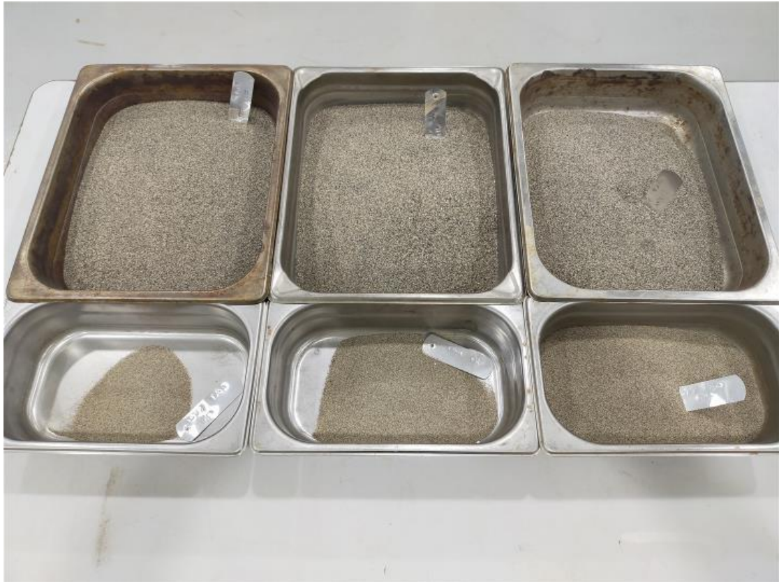
Plate 2 – Industrial sand from large scale pilot plant operation tested for asphalt and concrete applications
