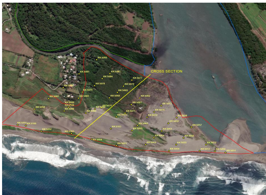
Figure 3 - Kulukulu South area, indicating the location of the cross-section shown in Figure 4. Note also the sand and gravel deposits filling the Sigatoka riverbed that will be dredged during the desilting project.
