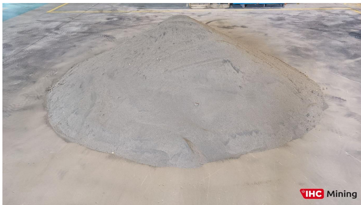
Plate 1 – “Run of mine” magnetite bearing industrial sand sample prepared for pilot plant processing
