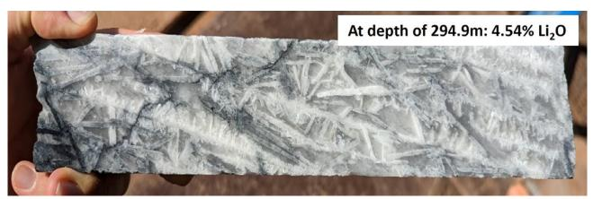
Figure 6: High-grade lithium samples from hole ANDD0208 within 22.8m @ 3.57% Li<sub>2</sub>0
