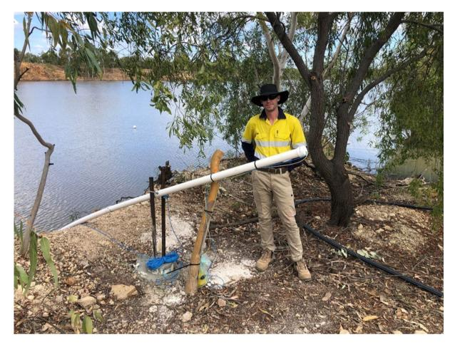
Figure 33: Installing 'Level Logger' water depth measuring equipment at Yandan Main Pit.
