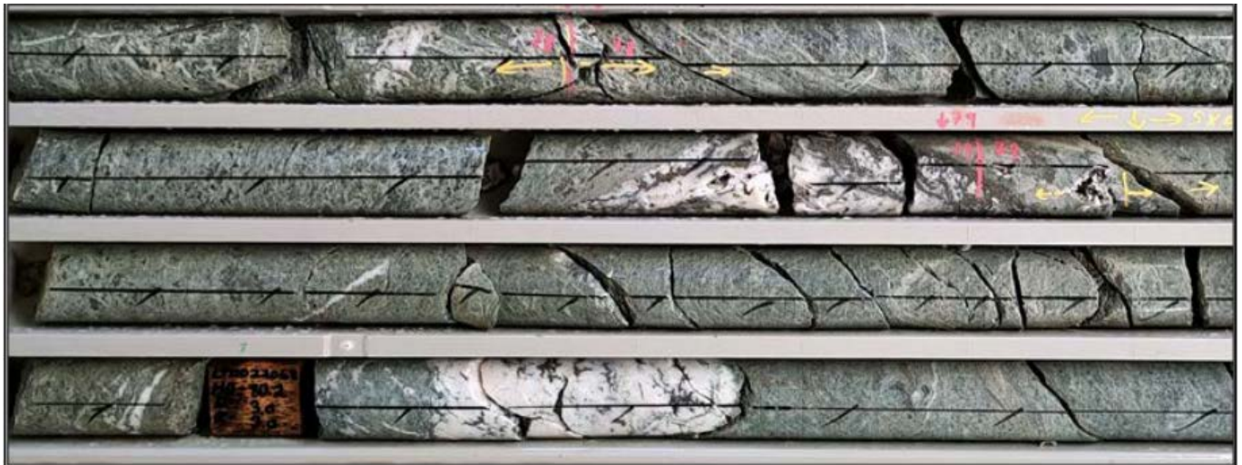
Figure 4. Gold and sulphide bearing quartz-barite veins in a zone which returned 8.5m @ 5.47g/t Au and 0.4% Cu (LTDD22068).
