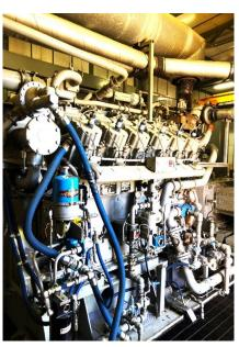
Part of the newly acquired RPGP – low pressure gas is compressed to sales gas pressure using gas engine driven reciprocating compressors
