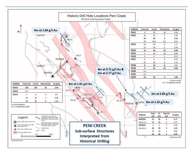
Figure 10: Sub-surface Structures (blue dashed lines) from Historical Drilling Results
