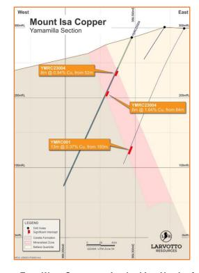
Cross-section looking N-W of IXL drilling of the targeted mineralization
