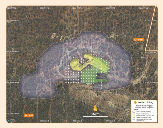
Figure 3. Munda optimised pit outline, starter pit and existing trial pit with proposed 10m x 10m pattern grade control drill holes.
