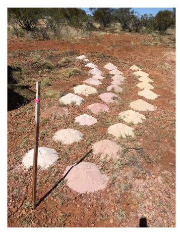
Aircore drilling was carried out at Crystal Creek during 2023 to test the tenor and extent of mineralisation, with a total of 32 drillholes for 541 metres completed during August. Thick intervals of prospective kaolinitic clays were encountered in many holes, and assay data were received from the laboratory during Q4 2023, with significant assay results summarised in the quarterly report released to the ASX on 31 January 2024.
