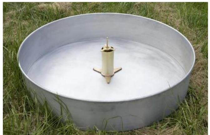
The tank type is a "Class A". This is a cylindrical galvanized sheet tank, 1.21 m in diameter and 25 cm deep. It is placed on a 10 cm high wooden platform, perfectly horizontal. The volume of water needed to maintain the constant level is measured, in the unit of time, which can be 6, 12 or 24 hours. The volume
