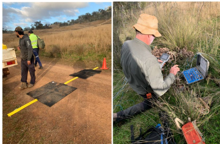
Figure 8 (L) and (R): Laying cabling, the main cable with road protection (L), geophysicist recording dipole readings (R)
