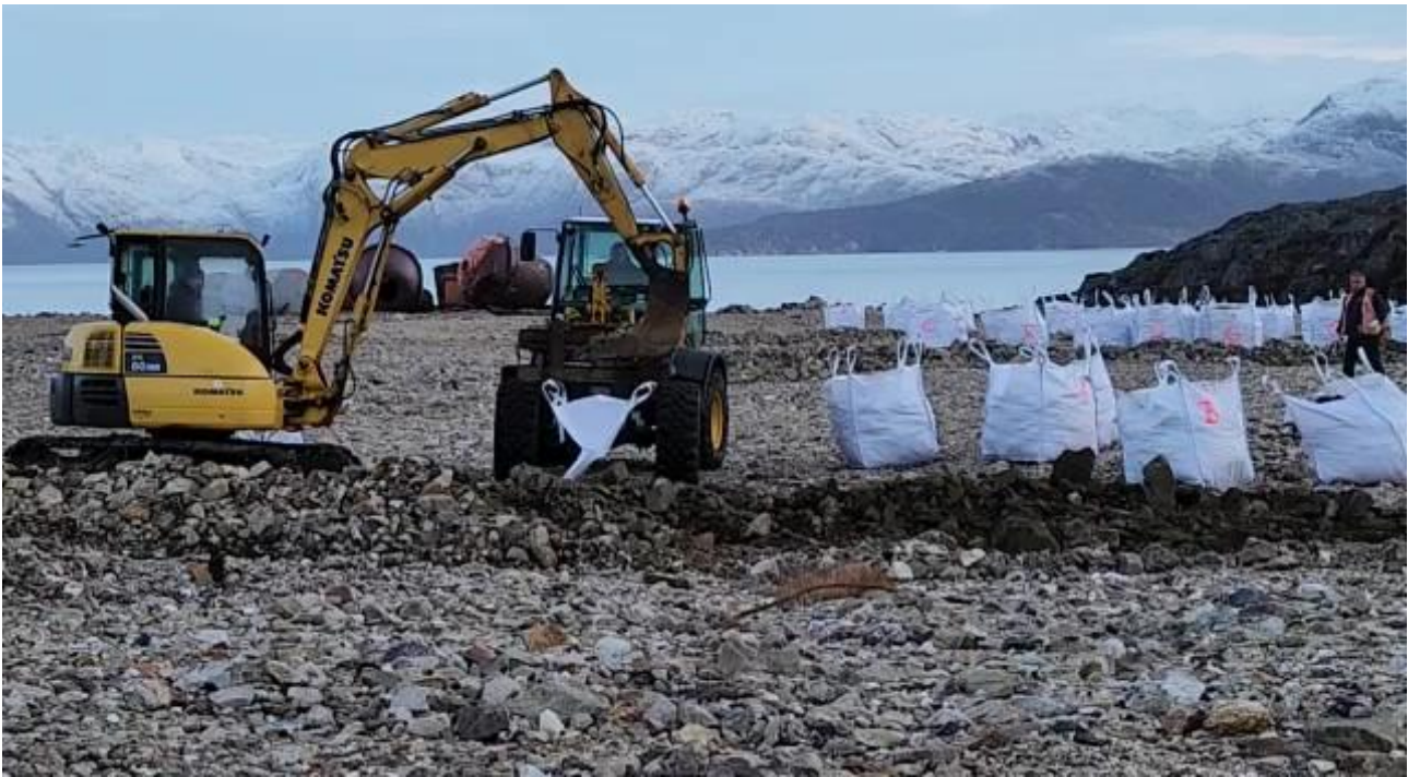
Figure 17: Collecting several tonnes of bulk samples from 5 trenches in the mineralized dumps.
