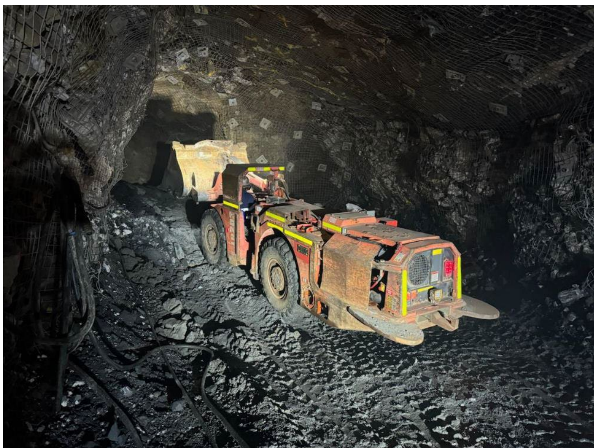
Figure 2: Cream Mining loader cleaning development headings at Paulsens underground.
