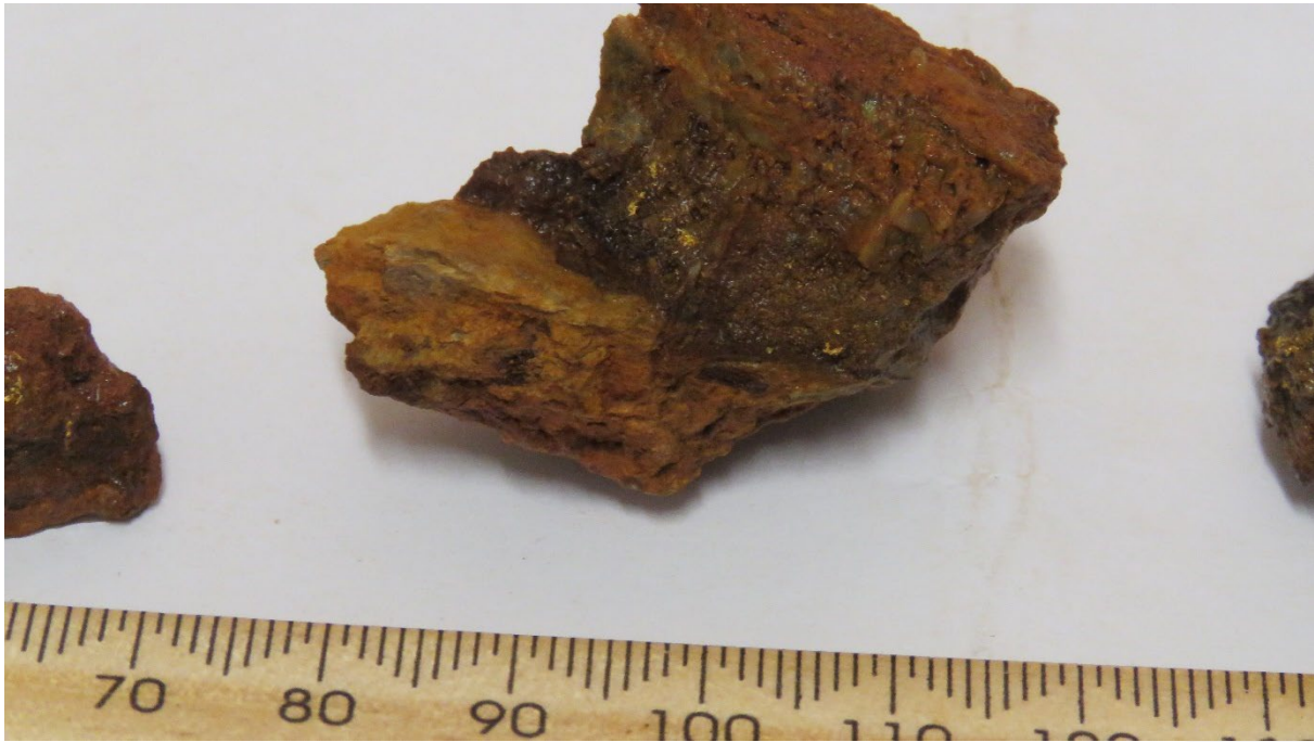
Figure 6: Samples from DPGM showing coarse visible gold
